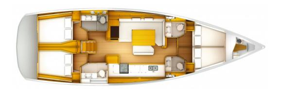
Shipyard: Jeanneau **Engine:** 75 HP Launched: 2016 Fuel tank: It. 240 Length overall: 15.38 m Water Tank: It. 615 Length of the hull: 14.98 m Berths: 8 + 3Width: 4.69 m Cabins: 4+1 skipper Draft: 2.28 m Salon: convertible
