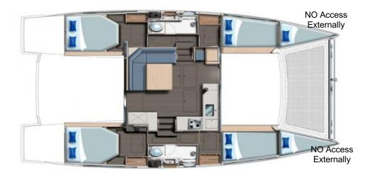
Shipyard: **Robertson and Caine** Engine: 2 x 29 HP 2019 Year: **Fuel Capacity:** 360 It 11.99 m Length overall: 780 It Water Capacity: Waterline Length 11.62 m 10 max Berths: Width: 6.72 m Cabins: 4 Draft: 1.25 m Bathrooms: 2 Sail Area: ca. 96 m<sup>2</sup>
