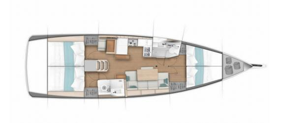
shipyard: **JEANNEAU 57 HP** engine It. 200 launched: 2019 fuel tank It. 530 length over all: 13.00 m drinking water tank: length of the hull: 12.64 m berths: 8 + 2width: 4.26 m cabins 4 draft: 1.60 m salon: convertible
