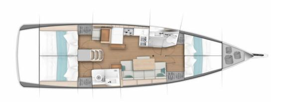
shipyard: **JEANNEAU** launched: 2020 13.00 m length over all: 12.64 m length of the hull: width: 4.26 m draft: 2.24 m ca. 90 m<sup>2</sup> sailarea:
