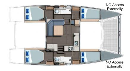
**Robertson and Caine** Shipyard: Engine: Year: 2018 Fuel Capacity: 11.99 m Length overall: Water Capacity: Waterline Length 11.62 m Berths: Width: 6.72 m Cabins: Draft: 1.25 m Bathrooms: ca. 96 m<sup>2</sup> Salon: Sail Area: Mainsail halfsticked with lazyjack and lazybag **Furling Genoa**
