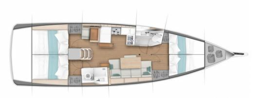
engine **57 HP** shipyard: **JANNEAU** fuel tank It. 200 launched: 2019 drinking water tank: It. 530 length over all: 13.00 m berths: 8 + 2length of the hull: 12.64 m cabins width: 4.26 m salon: convertible
