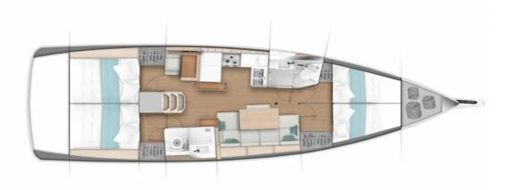
shipyard: JEANNEAU launched: 2019 length over all: 13.00 m length of the hull: 12.64 m width: 4.26 m draft: 1.60 m sailarea: ca. 90 m²
