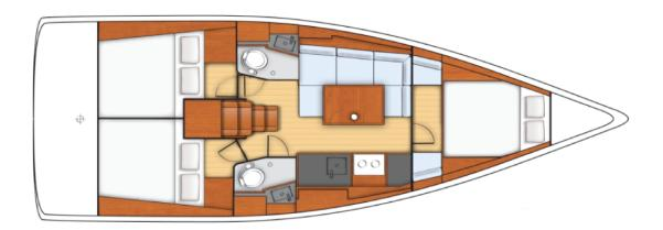
shipyard:Beneteauengine29 HPlaunched:2016fuel tanklt.130length over all:11.50 mdrinking water tank:lt.130+200ltlength of the hull:11.13 mberths:6 + 2
