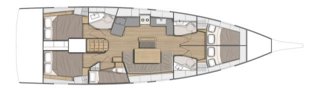
shipyard: Beneteau 80 hp engine launched: It. 200 2021 fuel tank length over all: 14.60 m drinking water tank: It. 570 length of the hull: 13.65 m berths: 10 + 2width: 4.50 m cabins 5
