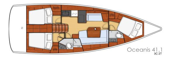
45 HP shipyard: Beneteau engine launched: 2017 fuel tank It.200 12.43 m length over all: drinking water tank: lt.570 length of the hull: 11.98m berths: 6+2 width: 4.20 m cabins draft: 1.68 m salon: convertible
