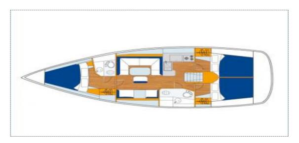
shipyard: Jeanneau launched: 2015 length over all: 12.34 m length of the hull: 11.00 m width: 3.99 m draft: 2.10 m
