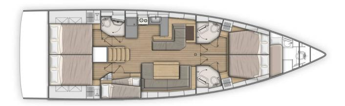
Shipyard: Beneteau 110 HP **Engine:** Launched: 2018 Fuel tank: It. 200 Length overall: 15.94 m Water Tank: It. 770 Length of the hull: 14.98 m 10 + 2Berths: Width: 4.80 m 5 + 1Cabins: Draft: 1.92 m Salon: convertible ca. 122 m<sup>2</sup> Sail Area: Heads: 3 + 1
