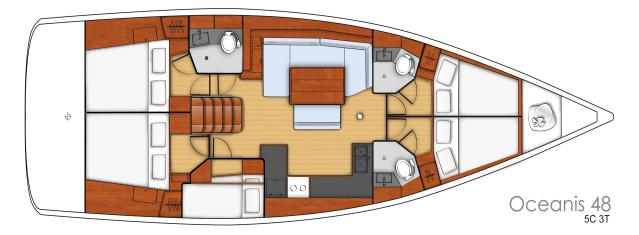
engine 75 hp shipyard: Beneteau fuel tank It. 240 launched: 2018 It. 690 drinking water tank: length over all: 14.60 m berths: 10 + 2length of the hull: 14.27 m cabins 5 width: 4.74 m
