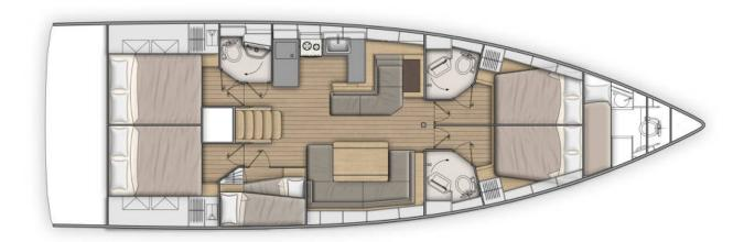
Shipyard: Beneteau **Engine:** 110 HP Launched: 2019 Fuel tank: It. 200 Length overall: 15.94 m Water Tank: It. 770 14.98 m Length of the hull: Berths: 10 + 2 Width: 4.80 m Cabins: 5 + 1 skipper Draft 1.92 m Salon: convertible ca. 122 m<sup>2</sup> Sail Area: Heads: 3 + 1 skipper
